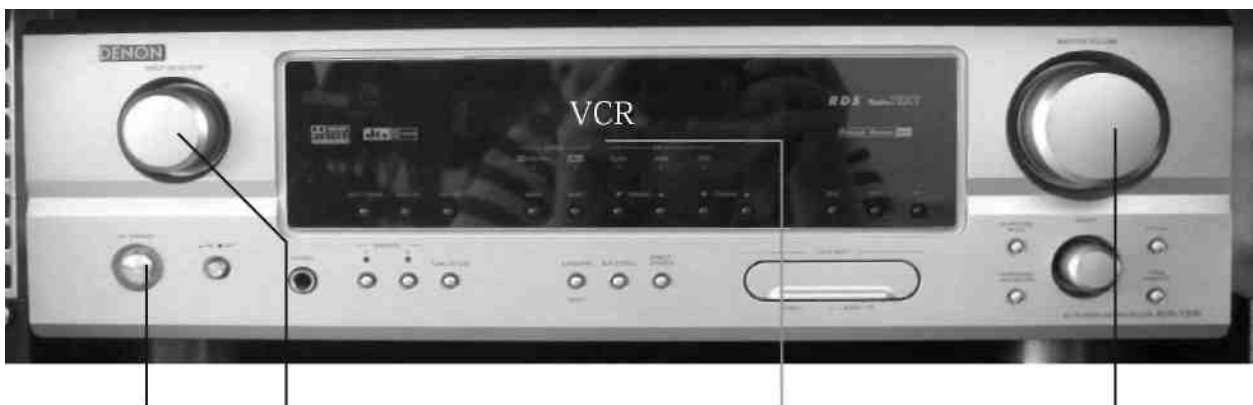
ON/STANDBY Input Selector Fig.3.2 VCR input Volume control
