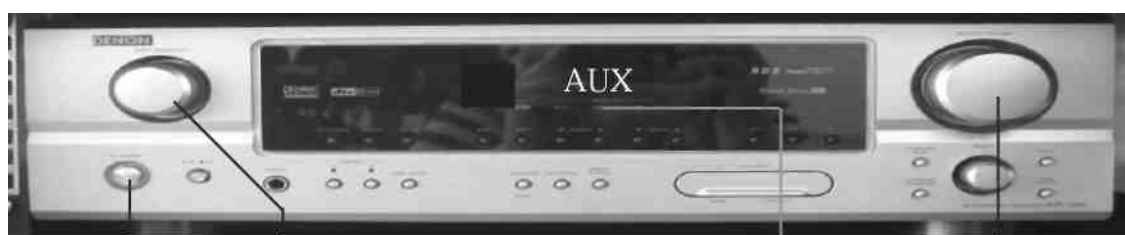
ON/STANDBY Function Fig.5.2 AUX input Volume control
